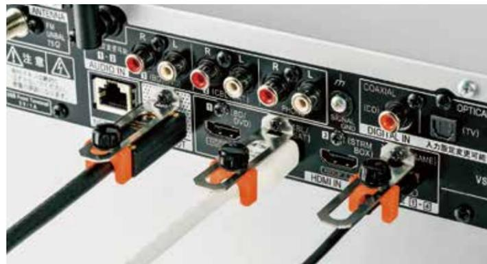
Has your HDMI cable attached to an AV receiver or other devices ever got disconnected or loose due to vibrations or unexpected accidents? The I/O Lock HDMI-WIDE can solve such problems. It can be easily attached to devices such as AV receivers that already have screws positioned above the HDMI port. As it uses the screws already attached to the device, no other alterations are necessary.
