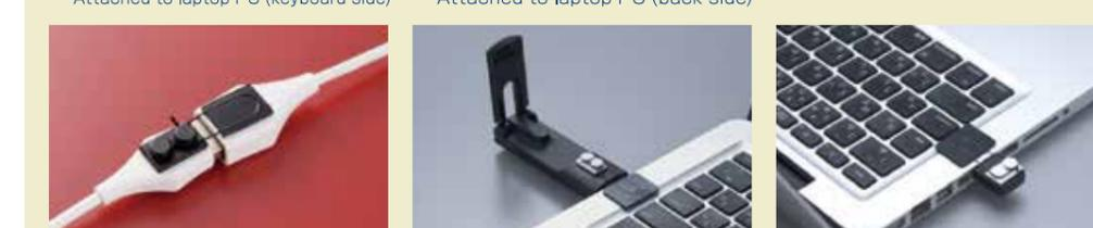
③USB の中継に取付 Attached to USB relay ④無線LAN 子機に取付 Attached to wireless LAN terminal ⑤小型無線LAN 子機に取付 Attached to mini wireless LAN terminal
